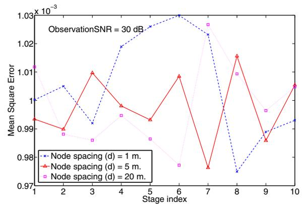
Fig. 1. The figure shows the plot of mean square error versus the stage index. We fix the observation SNR ( $\Gamma$ ) equal to 30 dB and assume the node spacing to be 1 m, 5 m and 20 m respectively.
