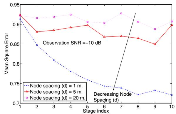
Fig. 2. The figure shows the plot of mean square error versus the stage index. We fix the observation SNR ( $\Gamma$ ) equal to  $-10$  dB and assume the node spacing to be 1 m, 5 m and 20 m respectively.
