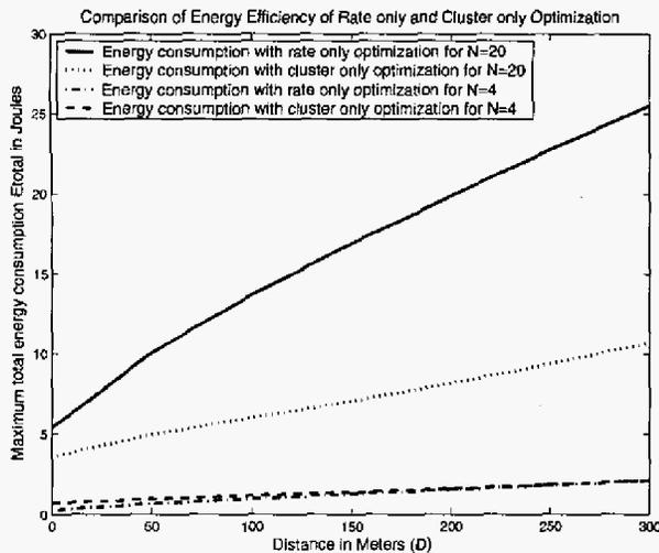
Fig. 2. The figure shows the comparison of optimized total energy consumption versus long haul distance for rate only and cluster only optimized transmission Schemes for  $N = 4$  and  $N = 20$  respectively.
