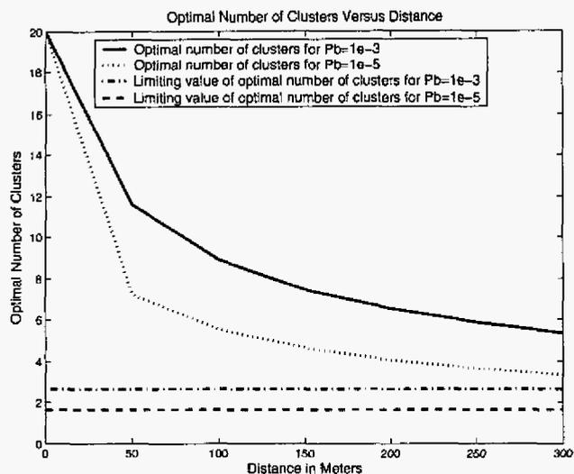
Fig. 1. The figure shows the plot of optimal number of clusters ( $K^*$ ) versus long haul distance ( $D$ ) for different values of probability of error ( $P_b$ ) and a given rate ( $b$ ).
