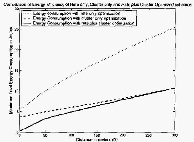
Fig. 3. The figure shows the comparison of optimized total energy consumption versus long haul distance for rate only, cluster only and joint rate and cluster optimized transmission Schemes for  $N = 20$ .
